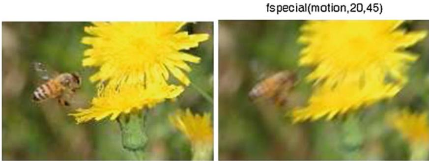
**Fig. 4.3** Lin. Convolution. filter of honey bee with Listing 4.4
